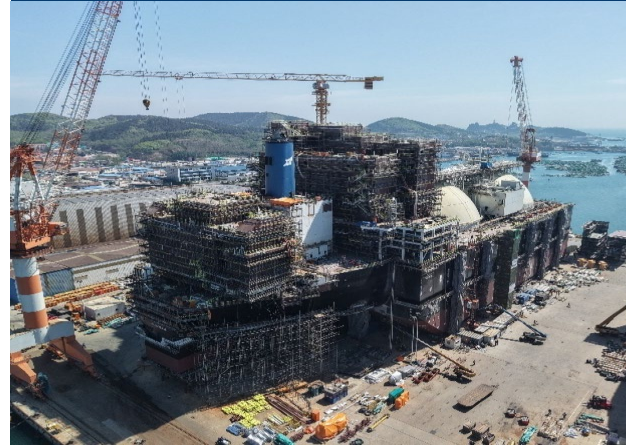
Midship fabrication status – all blocks installed
