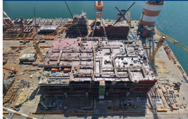
Midship fabrication status – all blocks installed
